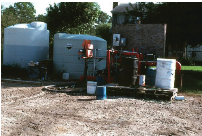
Figure 11. Injection system, fertilizer tanks, and computer control for drip irrigation.
