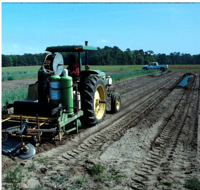
Figure 3. A combination mulch applicator that fumigates, presses the bed, and applies drip tape and plastic mulch in one pass. Credit: UF/IFAS
