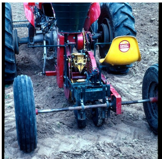
Figure 7. Direct-seeding through plastic mulch can be accomplished with this "plug-mix" planter. The machine punches a hole in the mulch and places a small amount of "soilless" mixture and seed into the hole.
