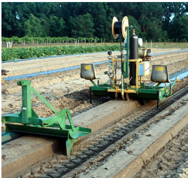
Figure 2. Bed press and mulch application machine (with drip tape attachment). Credit: UF/IFAS
