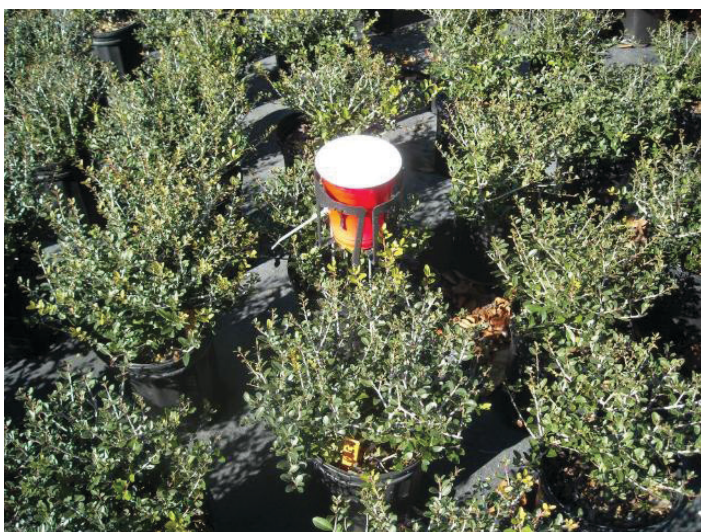
Figure 3. Irrigation collection cups are placed above canopy in the vicinity of test plants. Credits: Jeff Million
