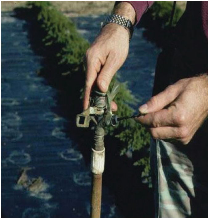
Figure 3. The blunt end of a drill bit with appropriate caliber is used to check orifice wear.
