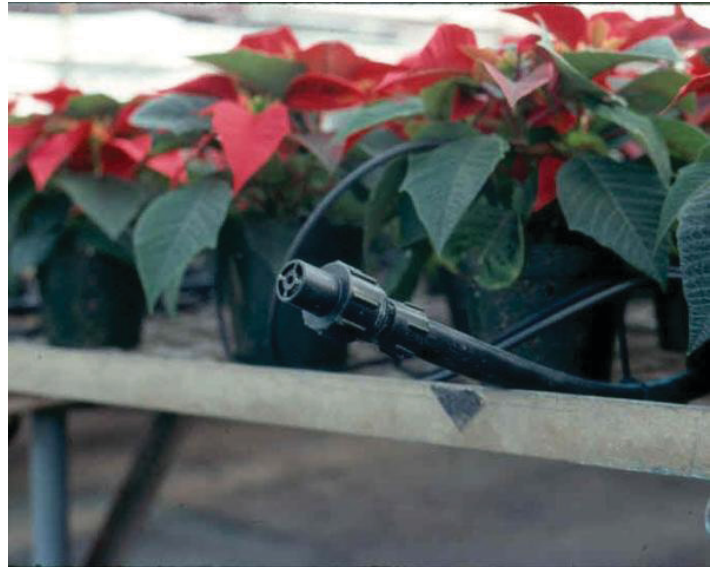
Figure 5. A low-pressure drain on the end of a pipe allows the pipe to drain rapidly when irrigation ceases.
