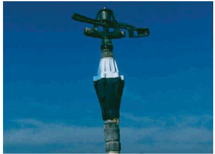
Figure 2. Appropriate nozzle operating pressure is achieved with a pressure regulator mounted below the sprinkler.
