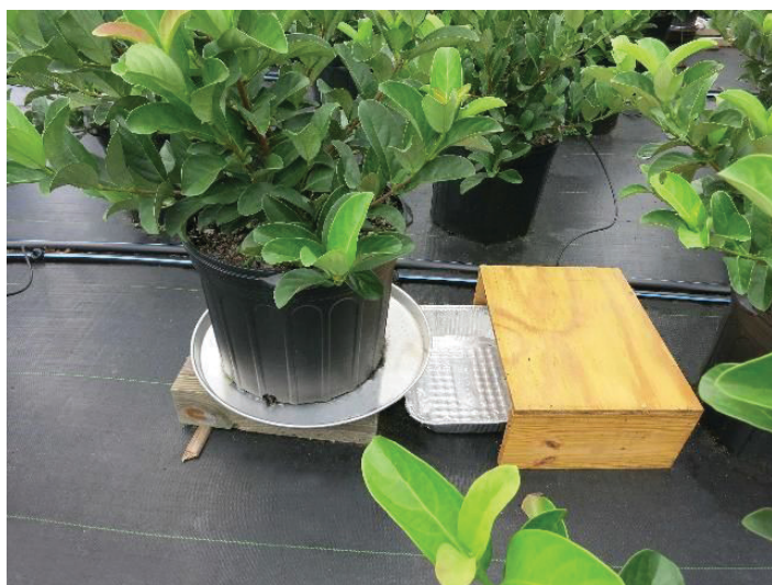
Figure 3. Microirrigated plants can be placed on a pizza pan raised several inches off the ground with pieces of 4x4 inch lumber. A drain hole punched out of the pizza pan allows leachate to drain into a tray for weighing. An emitter from an adjacent container is placed in a pail to determine the irrigation amount applied. This setup can remain in the field to facilitate routine testing. We often place a cover over the tray when collecting leachate during multiple irrigation cycles. Credits: Jeff Million, UF/IFAS
