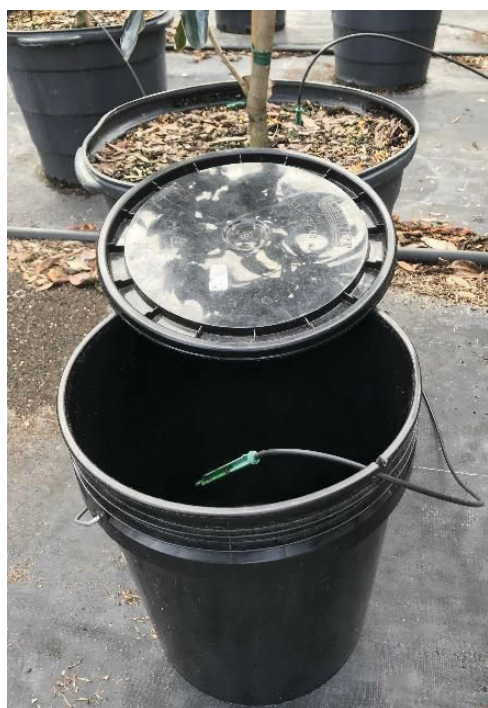
Figure 4. To determine the amount of spray-stake irrigation water applied during an LF test, an adjacent emitter is placed inside a pail. A notch cut into the lip of the pail prevents the emitter tubing from crimping when the lid is on. Credits: Jeff Million, UF/IFAS
