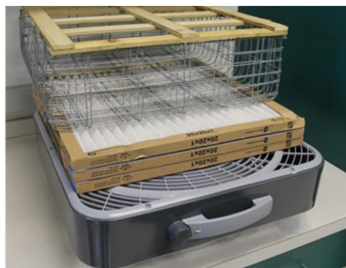
Figure 1. UF/IFAS MREC drying rig, spread out to show the possible components; From top to bottom: modified wooden slat, 20×20" wire cage, 20×20×1" natural fiber household air duct filters, 20" box fan. Credits: Sean M. Campbell, UF/IFAS
