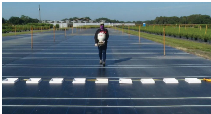
Figure 5. Calibrating a belly-grinder spreader by first determining swath width using collection pans.
