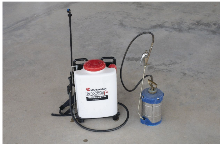
Figure 7. Backpack and smaller hand-held compression sprayers can be useful for spot-treating and even applying preemergence herbicides over the top of ornamentals in small areas.
