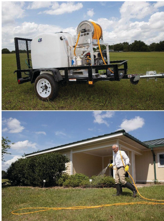
Figure 10. Skid sprayer systems are most commonly used by pest control companies and in turfgrass applications, but they can also be utilized by container nurseries for certain uses.
