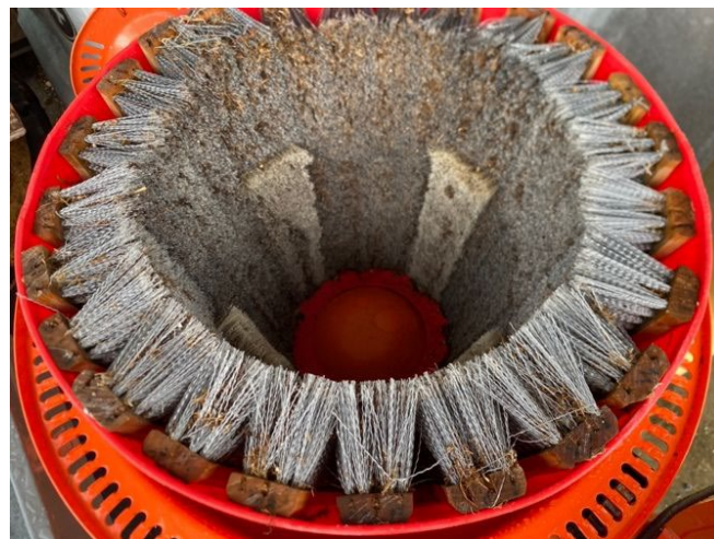
Figure 15. Once all the brushes are attached, there should be very little space between brushes and no gaps between brush bristles.
