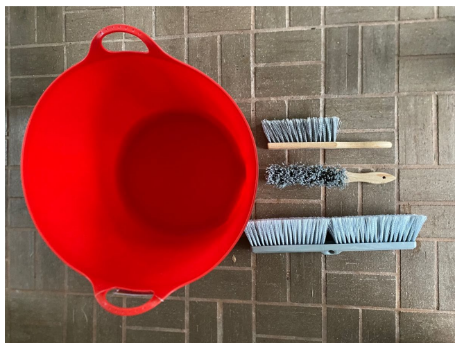
Figure 11. A flexible tub (left) can be used as a liner inside the concrete mixer, and alternative types of bench brushes or broom heads (right) can be cut and placed inside the liner.
