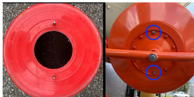
Figure 12. (Left) A large-diameter hole needed to be cut into the center of the tub liner to help it sit snugly on the bottom of this concrete mixer. (Right) The silver bolts attach the liner to the mixer base.
