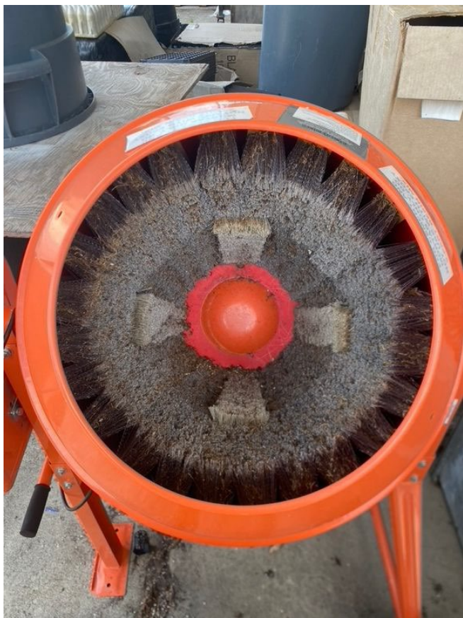
Figure 16. Looking into the finished barrel washer interior with the dome in place.
