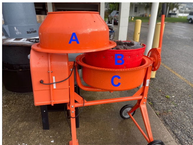
Figure 10. The mixer dome (A), flexible tub in place (B), and mixer base (C).
