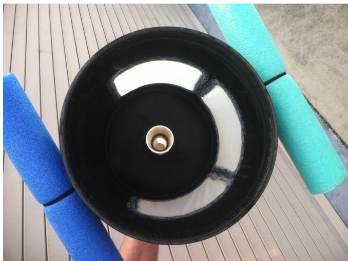
Figure 2. An internal view of the collection bucket portion of a floating airlift collector used at the UF/IFAS Tropical Aquaculture Laboratory. Credits: Jason S. Broach
