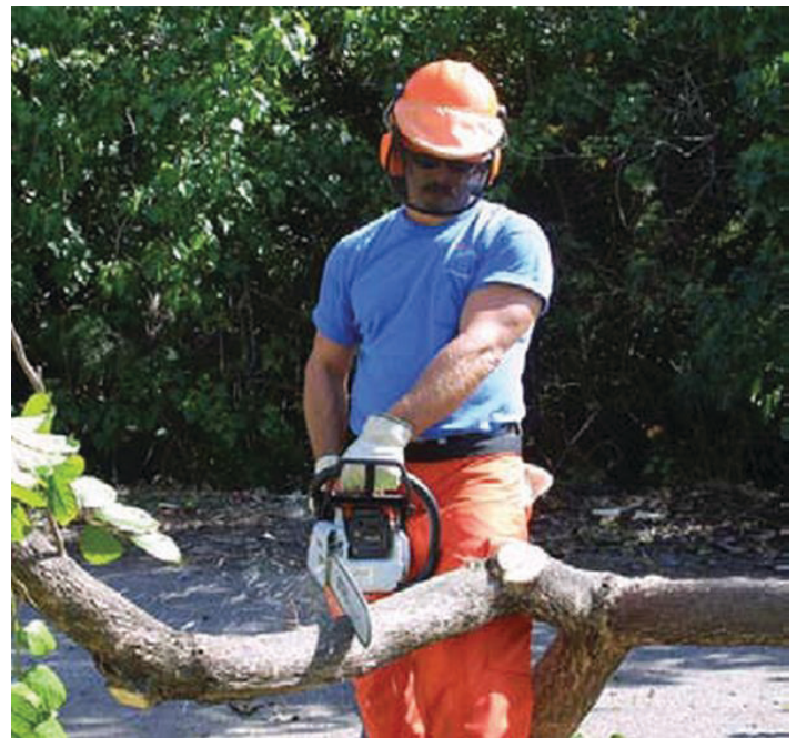
Figure 3. Cut at waist level or below to avoid injuries. Credits: 2003 Hot Pixel Press/Arbor Global LLC
