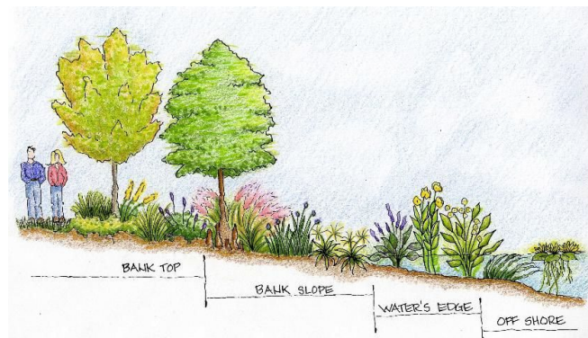
Figure 3. Illustration of stormwater pond planting zones along a moderate to gentle slope.
