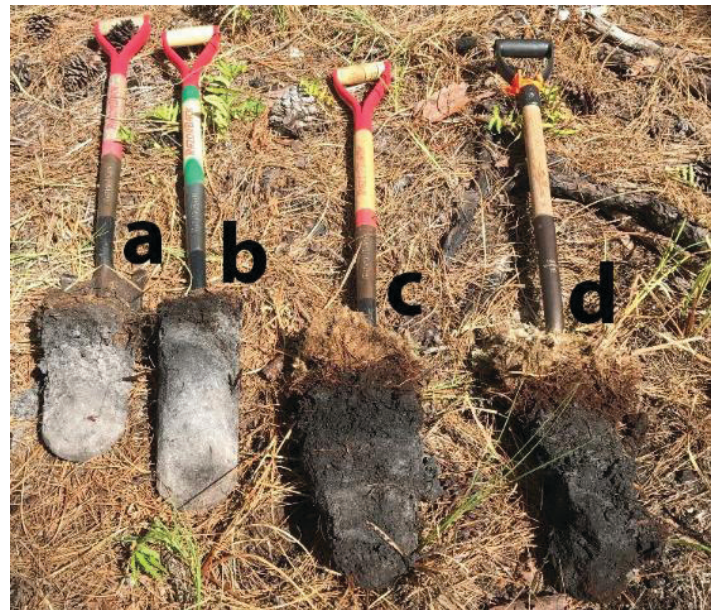
Figure 3. These soils were dug up along a topographic gradient in Gainesville, Florida. Soils a and b were higher in elevation compared to soils c and d. Subsequently soils c and d are darker in color due to increased organic matter content as a result of longer periods of inundation.
