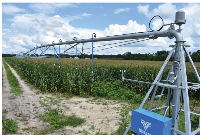
Figure 1. Center pivot irrigation system with low pressure drop nozzles increase crop water uptake efficiency.
