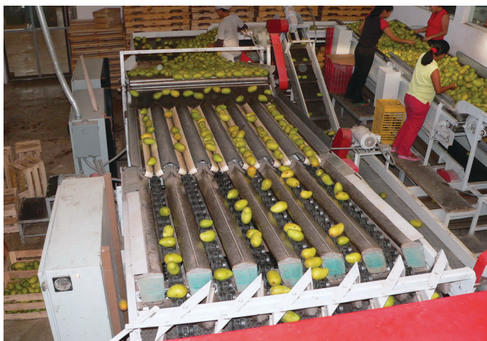
Automated fruit sizing on the packingline
