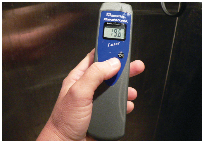
Measuring surface temperature with an infrared thermometer
