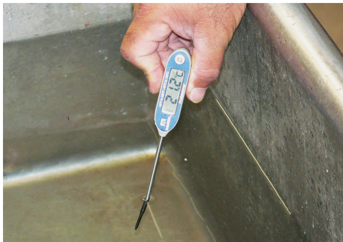
Measuring hydrocooler water temperature
