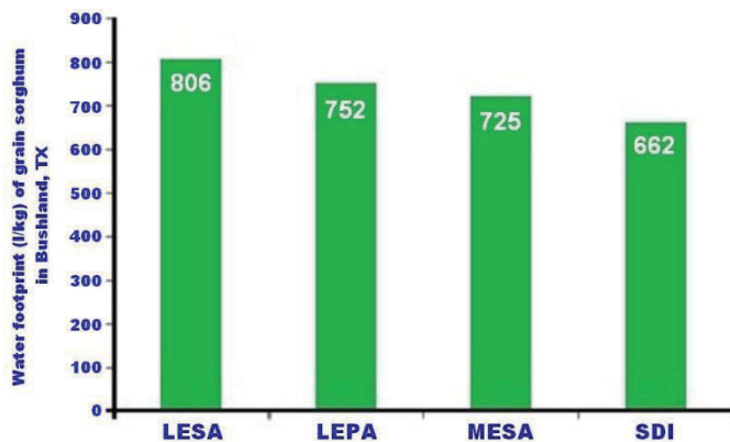
Figure 5. Significantly lower water footprints for sorghum under SDI compared to sprinkler irrigation were observed during 2000–2002 seasons in Bushland, Texas (Colaizzi et al. 2004).
