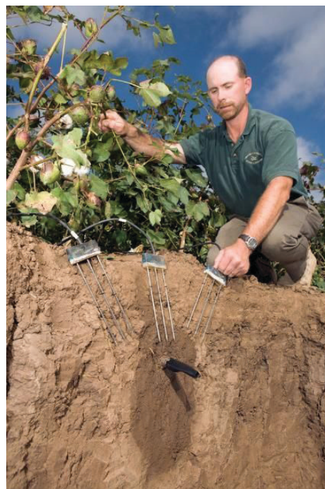
Figure 3. SDI placed deep in a cotton field allows for long lifetimes and avoids interference from tillage. Soil-water monitoring probes allow for measurement of soil moisture. Credits: Peggy Greb
