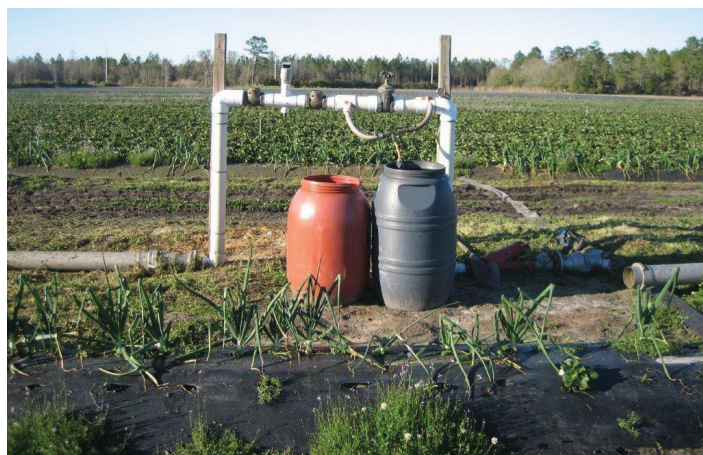
Figure 1. Fertigation unit for small acreage.
