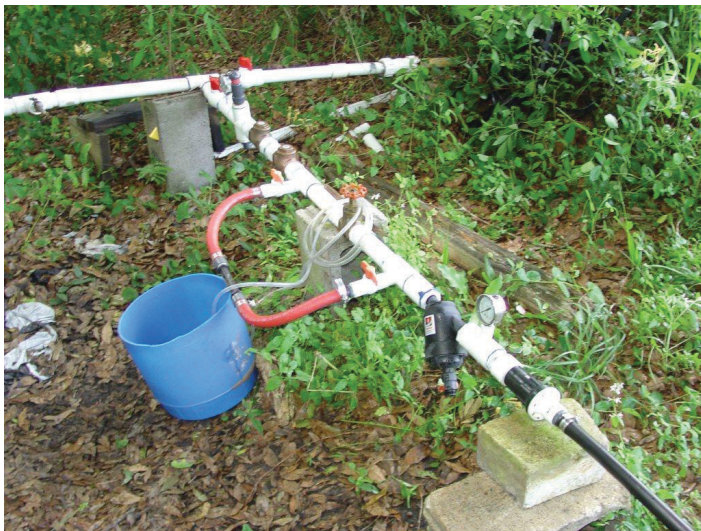
Figure 3. Fertigation assembly with proper backflow prevention and filtration.
