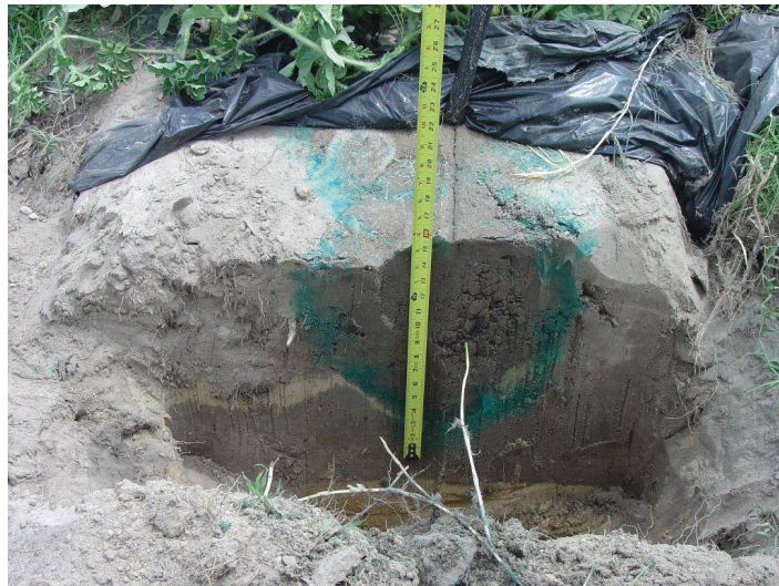
Figure 4. Using blue dye to demonstrate water movement in root zone after irrigation.
