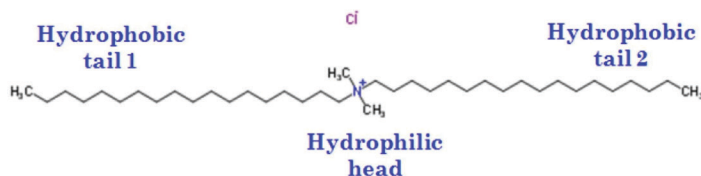
Figure 4. Chemical structure of a cationic surfactant, dimethyldioctadecylammonium chloride (DDAC). Its chemical formula is C_{38}H_{80}ClN . This surfactant has two 18-carbon hydrophobic tails and one positively charged nitrogen-hydrophilic head.
