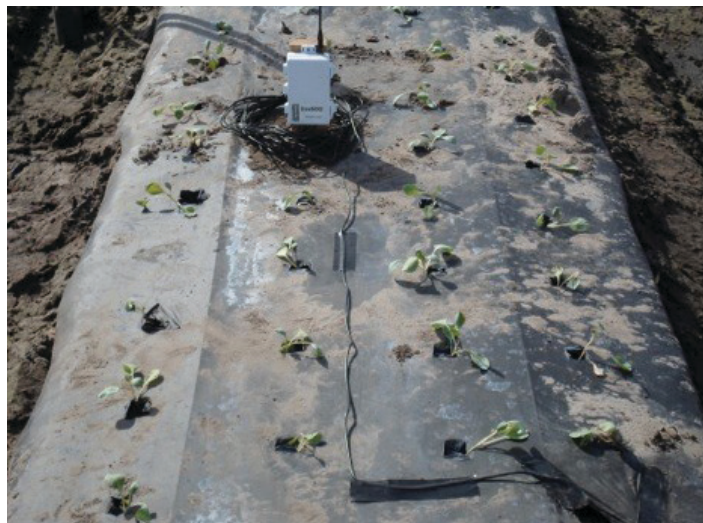
Figure 6. Soil moisture sensors installed under plastic mulch in both inner and outer plant rows.
