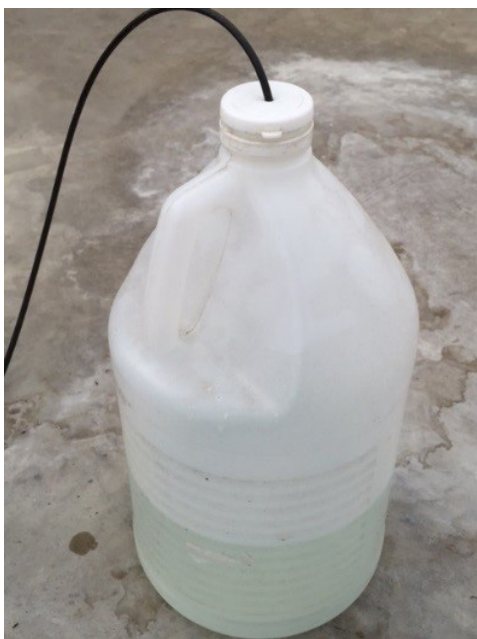
Figure 8. Gallon jug used to collect irrigation leachate. Credits: UF/IFAS
