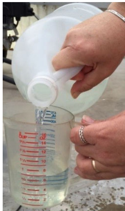
Figure 9. Measuring leachate volume. Credits: UF/IFAS
