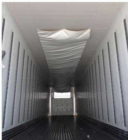
Figure 9. Interior view of refrigerated trailer showing flat sidewalls, duct extension, air delivery chute, pressurized return air air bulkhead, a duct extension, and an air delivery chute attached to the ceiling of a reefer trailer. (Source: PEB Commodities, Inc.)
