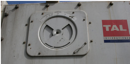
Figure 4. Picture illustrating manual fresh air exchange within a reefer container. (Source: PEB Commodities, Inc.)
