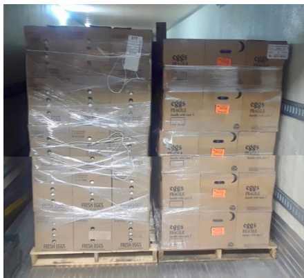
Figure 45. A palletized load of eggs. Stretch film is wrapped around the pallet loads to reduce the possibility of vibration damage, but is twisted once per side so as to not completely seal the pallet loads – avoiding potential moisture buildup. (Source: P.E. Brecht)
