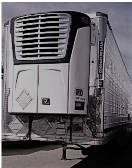
Figure 8. External view of trailer, refrigeration unit and insulated trailer. (Source: Thermo King)
