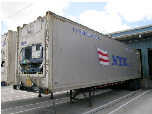
Figure 2. External views of refrigerated containers showing an integral refrigeration unit attached to an insulated container (box) and a chassis. (Source: PEB Commodities, Inc.)
