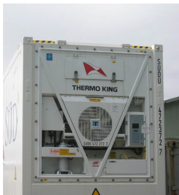
Figure 2. External views of refrigerated containers showing an integral refrigeration unit attached to an insulated container (box) and a chassis. (Source: PEB Commodities, Inc.)
