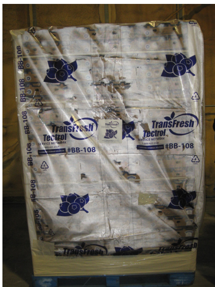
Figure 42. A pallet of blueberries, enclosed in an airtight plastic bag and injected with a modified atmosphere. (Source: S. Sargent)
