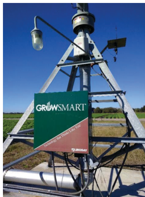
Figure 1. The head of a center-pivot irrigation system used for fertigation in southwest Florida.
