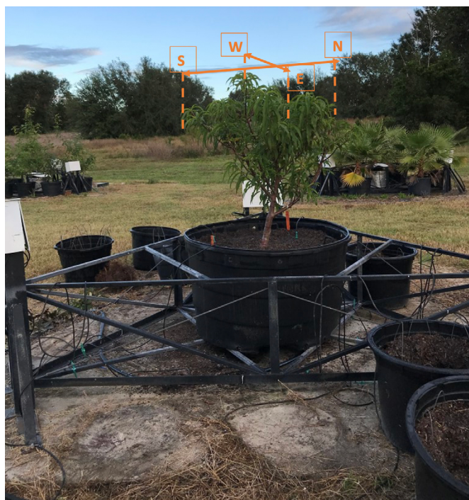
Figure 4. Weighing lysimeter used to determine the actual evapotranspiration (ETA) of young peach trees by weighting the volume of water is lost by evaporation and transpiration daily. The yellow arrows indicate the projected canopy area measurements in feet.
