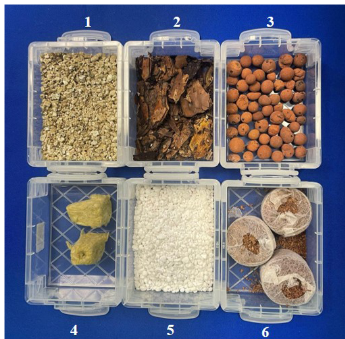
Figure 3. Examples of growing media for small hydroponics: vermiculite (1), composted pine bark (2), LECA (3), rockwool (4), perlite (5), and coconut fiber (6). Credits: Jonael Bosques, UF/IFAS
