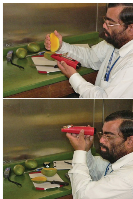
Figure 34. Measuring mango fruit SSC with a refractometer.
