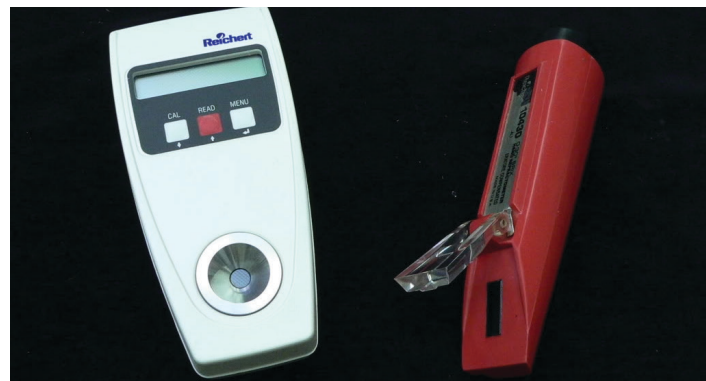
Figure 33. Handheld digital scale (left) and visual scale (right) refractometers.
