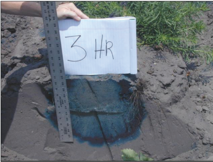
Figure 3. Cross section after 3 hours of irrigation. Credits: J. R. Duval (2002)
