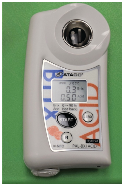
Figure 2-10. A portable titrimeter/refractometer for measuring soluble solids and acidity of juice.
