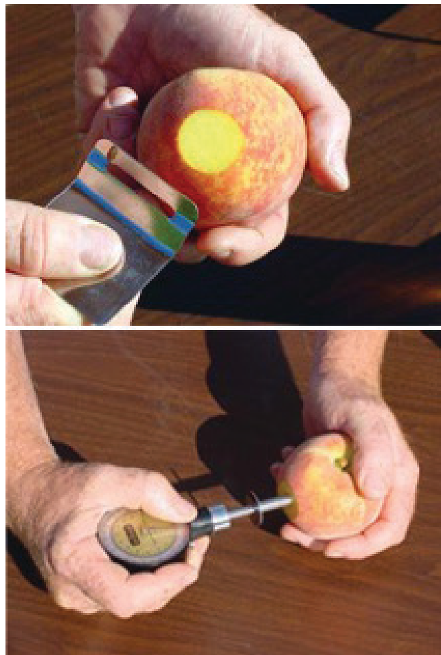
Figure 2-8. Measuring fruit firmness with a penetrometer. A portion of the peel must be removed before taking the measurement.
