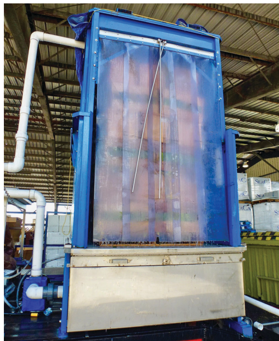
Figure 8-8. A stationary (batch) hydrocooler, which runs for a predetermined time to achieve \frac{7}{8} cooling.
