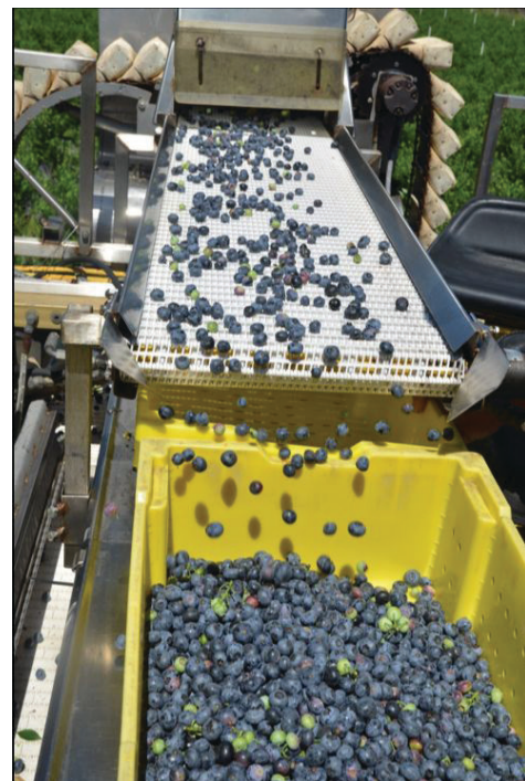
Figure 4. Harvester conveyor emptying blueberries into fruit lugs. Credits: Jeff Williamson, UF/IFAS
