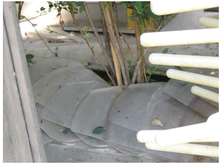
Figure 3. Harvester catch plates closing around plant crown. Credits: Jeff Williamson, UF/IFAS
