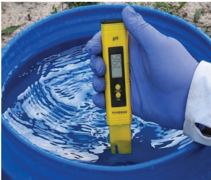
Figure 8. Measurement of the source water's pH before adding any acid.
