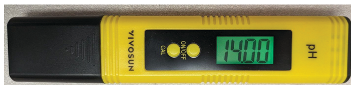
Figure 2. A digital pH meter suitable for measurements of irrigation water in the field.
