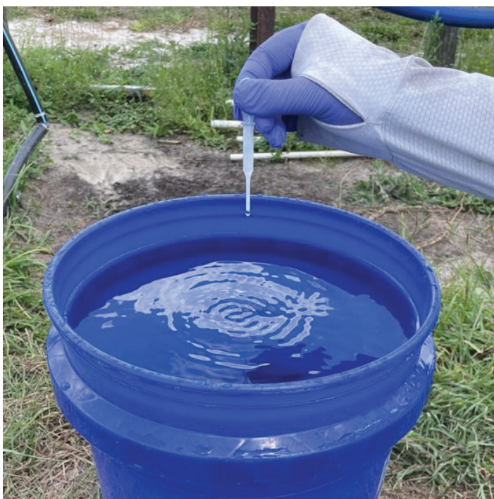
Figure 9. Adding drop by drop of 10% sulfuric acid to the irrigation water in a 5-gallon bucket.
