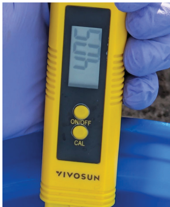
Figure 10. Measurement of the source water's pH after adding 10 mL of 10% sulfuric acid.
