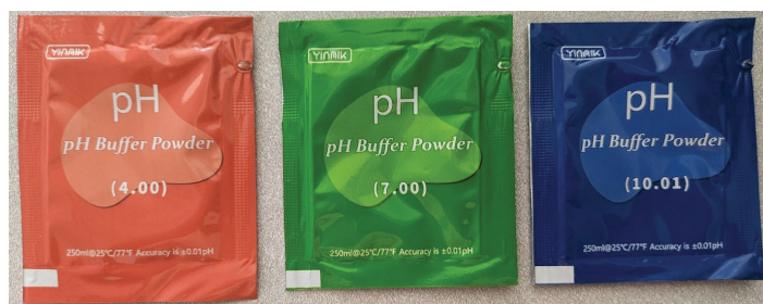
Figure 3. A set of pH buffer powders for pH calibration. The colors represent the standard pH values: red stands for pH 4.00, green for pH 7.00, and blue for pH 10.01. This set of pH buffer powders is commercially available online.
