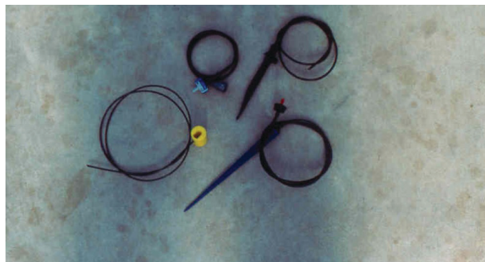
Figure 18. Various irrigation emitters, including button emitters and spray stakes.
