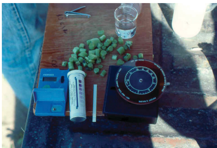
Figure 12. Plant petiole sap-testing kits for measuring nitrogen status of plants.
