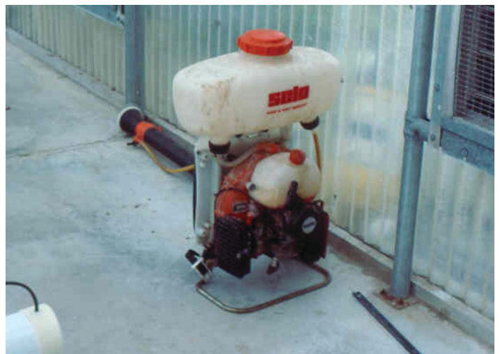
Figure 31. Motorized, backpack sprayer for applying pesticides.
