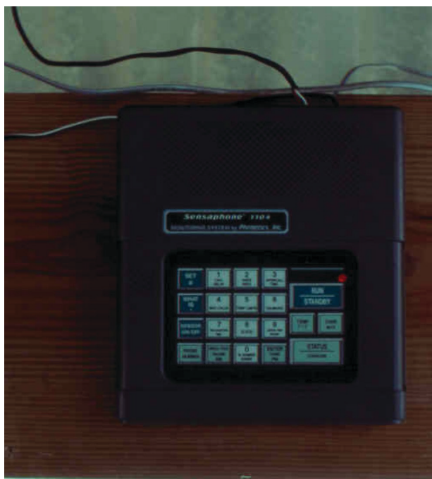
Figure 24. Alarm device that phones owner of deviations in set environmental parameters.
