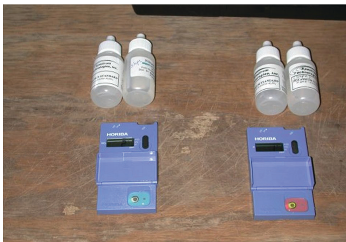
Figure 2. Sap testing for vegetables involves separating the petiole from the leaf blade, (2.1) calibrating the nitrate ( \text{NO}_3\text{-N} ) and potassium (K) ion specific electrodes (Cardi meter shown here) with standard solutions, (2.2) extracting the sap, (2.3) collecting the sap from the press, and (2.4) placing a droplet of sap on the electrode. A hydraulic press may be needed only when few petioles are available or when petioles contain little sap as may occur with strawberry. In most cases, a garlic press will be an adequate tool to extract the sap. Readings should be compared to published sufficiency ranges.
