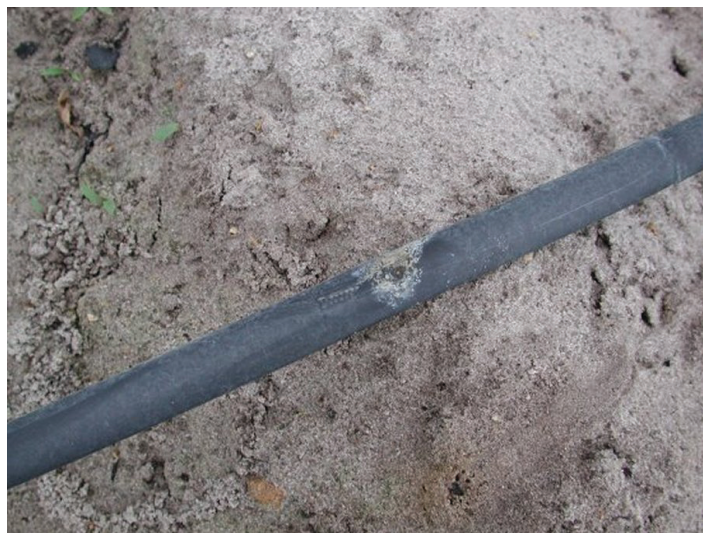
Figure 7. Accumulation of precipitates around a drip-tape emitter (8.1) may result in an uneven water distribution pattern (8.2).
