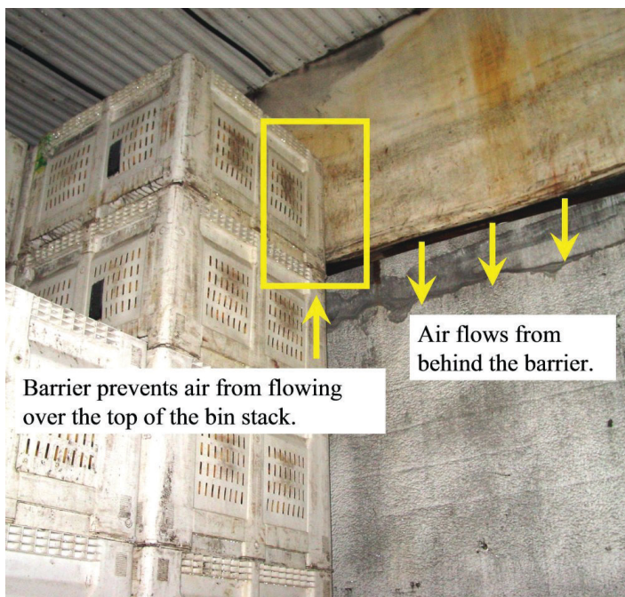
Figure 3. Bin stacked to prevent air from flowing over the top.
