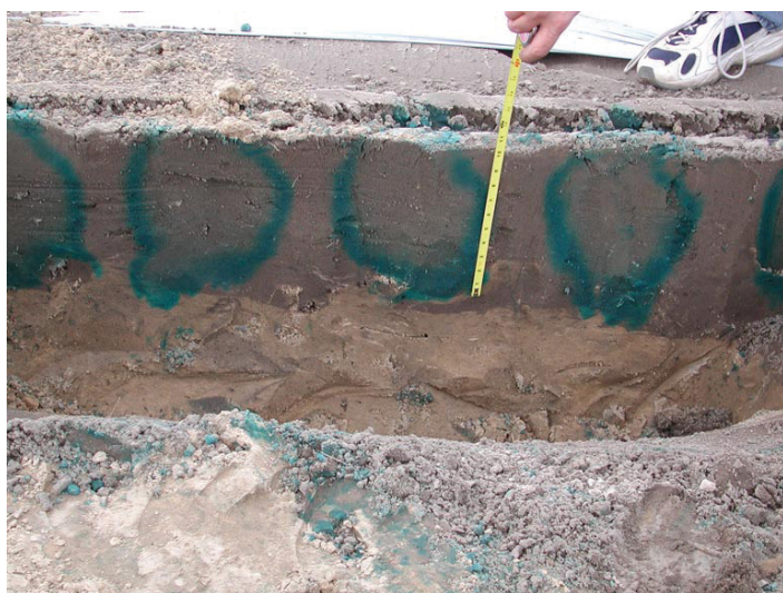
Figure 3. A wetted zone after 1hr irrigation using a 24 gal/100ft/hr drip tape on a Blanton Alpine Foxworth fine sand near Live Oak, FL.
