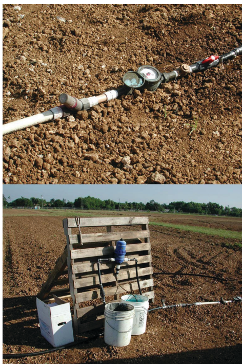
Figure 1. Injection system used for the dye test on a Krome very gravelly loam at the UF/IFAS Tropical Research and Education Center in Homestead, FL.
