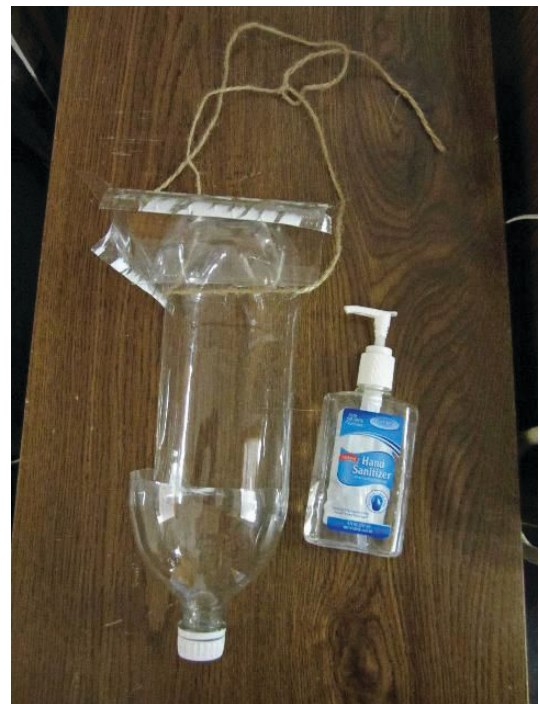
Figure 20. Bark and ambrosia beetle ethanol trap made from soda bottle with a large “window” and hand sanitizer. Credits: Adrian Hunsberger, University of Florida
