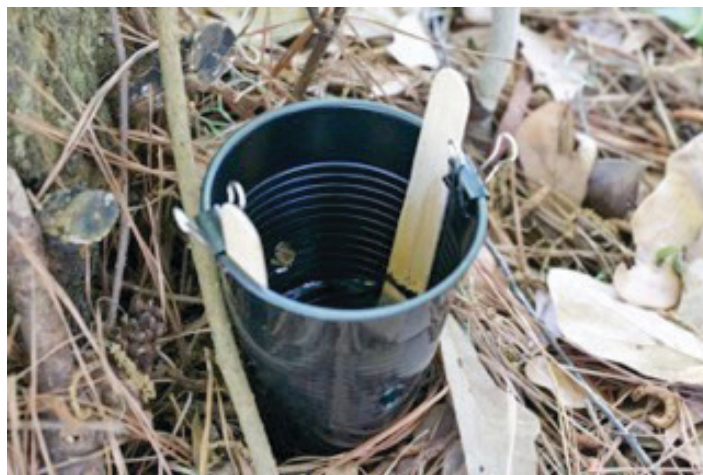
Figure 5. Standard ovitrap used for monitoring Aedes aegypti and Aedes albopictus .
