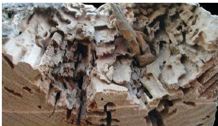
Figure 19. Neotermes jouteli (Banks) damage in 4-inch x 8-inch beam removed from a house in Ft. Lauderdale. Credits: Rudolf H. Scheffrahn, UF/IFAS
