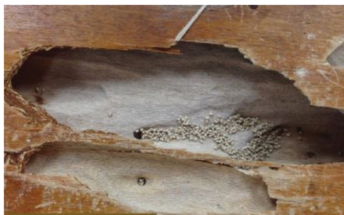
Figure 21. Drywood termite galleries are smooth, going across the grain of the wood, and can be several feet long. Credits: Faith Oi, UF/IFAS
