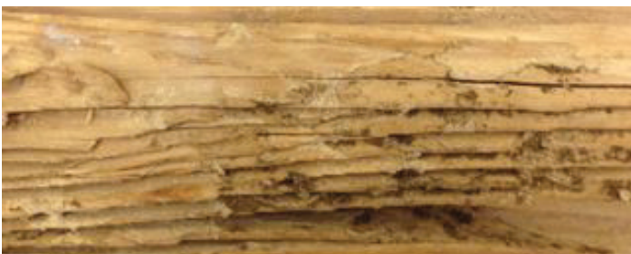
Figure 28. Subterranean termite feeding damage along the grain of the wood. Credits: Faith Oi, UF/IFAS
