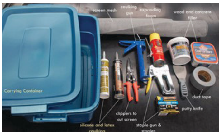
Figure 11. Sample equipment needed for bee-proofing. Credits: UF/IFAS Honey Bee Lab
