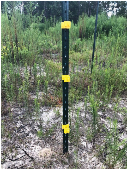
Figure 4. Insulators at 8 inches (0.2 m), 20 inches (0.51 m), and 32 inches (0.81 m). Credits: K. Post, UF/IFAS
