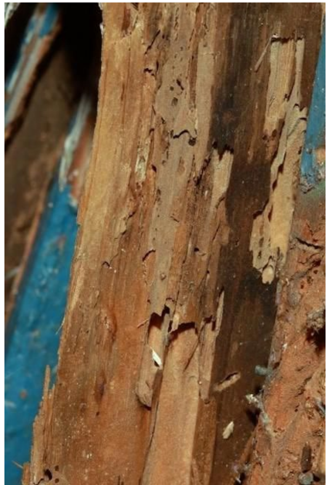
Figure 11. Wood damaged by Cryptotermes brevis (Walker). Credit: Johnalyn M. Gordon, UF/IFAS
