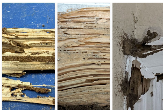
Figure 9. Feeding damage from Coptotermes subterranean termites (right) and feeding damage with soil in galleries (left).
