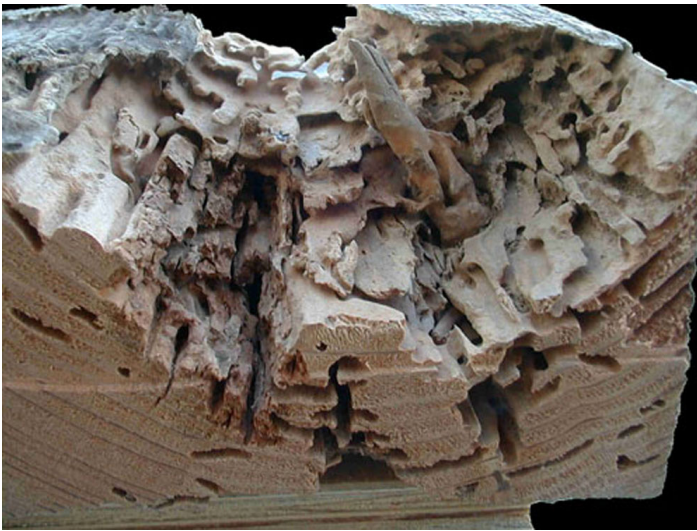
Figure 17. Neotermes jouteli (Banks) damage in 4-inch x 8-inch beam removed from a house in Ft. Lauderdale. Credits: Rudolf H. Scheffrahn, UF/IFAS
