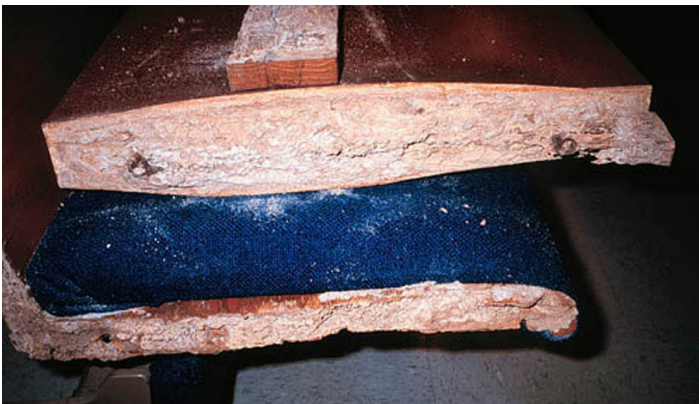
Figure 9. Damage by Coptotermes gestroi (Wasmann) to church pew, Miami.
