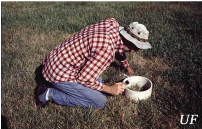
Figure 3. Using the flotation method to monitor for the southern chinch bug, Blissus insularis Barber.
