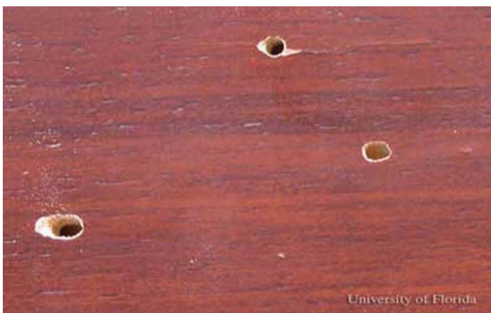
Figure 5. Exit holes for adults of Heterobostrychus aequalis (Waterhouse), a wood-boring beetle. Credits: Lyle J. Buss, UF/IFAS
