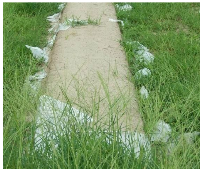
Figure 5. Breakdown of plastic film caused by prolonged sun exposure.
