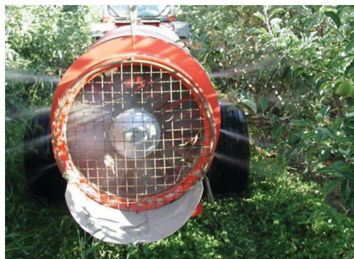
Figure 6. Applying entomopathogenic nematodes in an orchard using tractor-mounted airblast sprayer configured for this purpose. Credits: Lawrence Lacey, USDA
