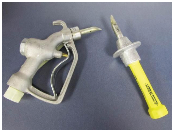
Figure 2. Varieties of pressure-rinse nozzles. Credits: UF/IFAS
