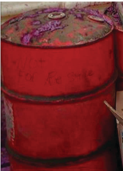
Figure 1. Pesticide drum bulging from extreme heat.
