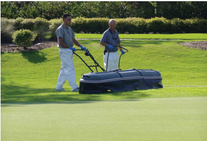
Figure 16. Shielded sprayer application to a golf course green. Credits: UF/IFAS Pesticide Information Office
