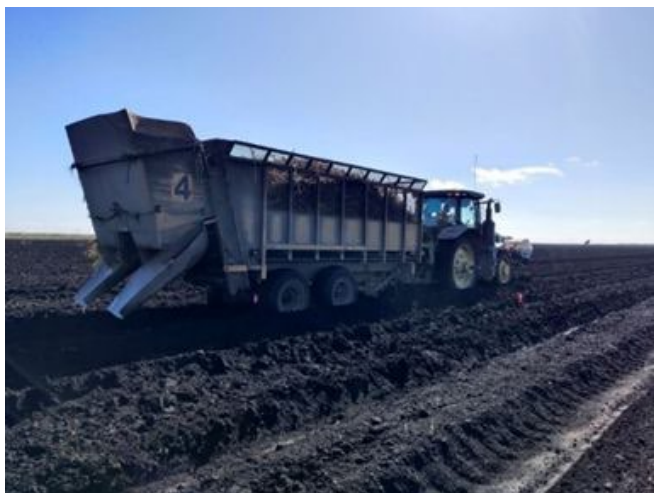
Figure 3. Rear planting elevator-style mechanical planter with chute-mounted nozzles.
