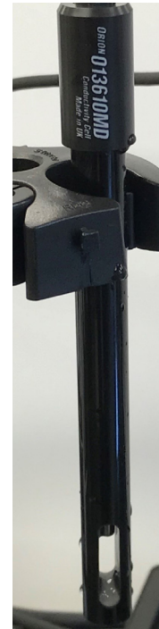
Figure 3. Graphite cell with 4-electrode-Epoxy sealed.
